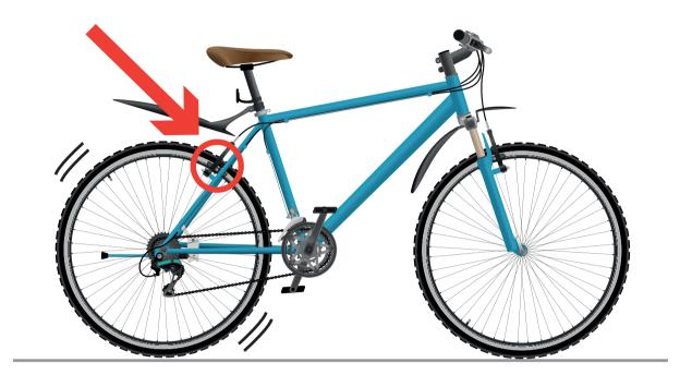
Pulling only the back brake causes the back wheel to skid, but will not stop the bike traight away
