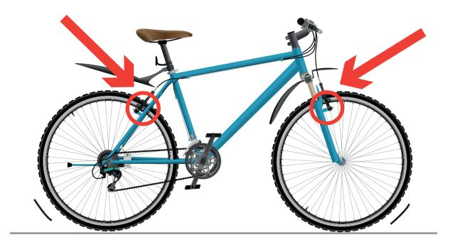
Pulling both brakes, back just before the front, should stop bike smoothly and quickly
