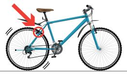
Pulling only the back brake causes the back wheel to skid, but will not stop the bike straight away
