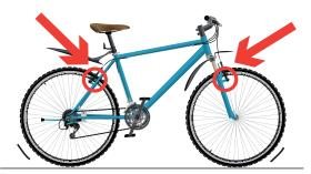
Pulling both brakes, back just before the front, should stop the bike smoothly and quickly
