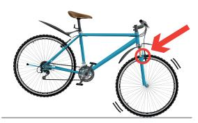
Pulling only the front brake will cause the front wheel to stop and the back wheel to lift off the ground
