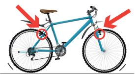
Pulling both brakes, back just before the front, should stop the bike smoothly and quickly
